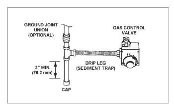
FIGURE 19. GAS PIPING WITH FLEXIBLE CONNECTOR.
